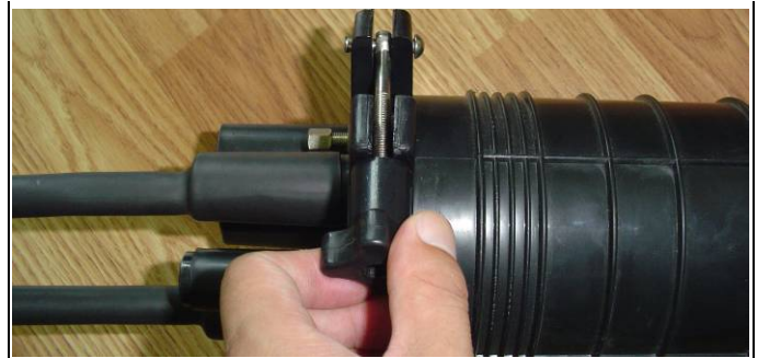
(17) Put on the clamp, run the ferris wheel to fix the base and barrel.
