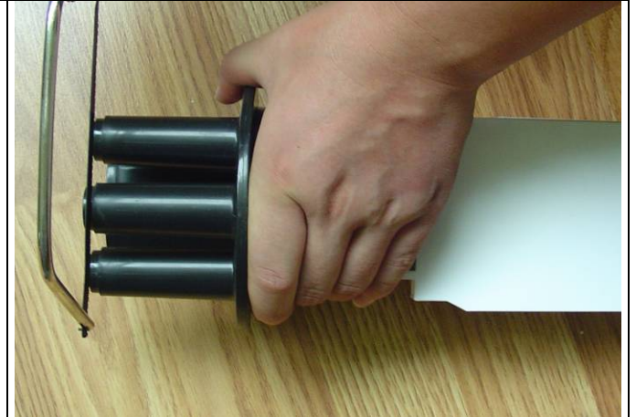
(1) Saw the entry ports as need.
