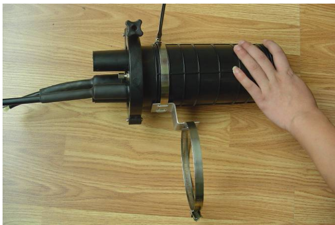
(18) When installing, fix the hanging hook as showing. Fix the closure with steel belt by minus screwdriver, and, fix another steel belt on the aerial-hanging pillar.
